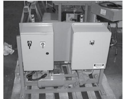
Lubricated/cooling oil units
